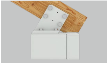
side view eaves fixture
