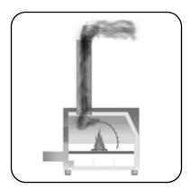
Generic flue system allows the heat and flame to escape the oven chamber immediately requiring more time to reach desired temperatures.
