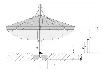
Loose cover max. 10 cm, concrete thickness min. 30 cm (pay attention to frost depth), Guarantee water drainage, Supply line electric.
